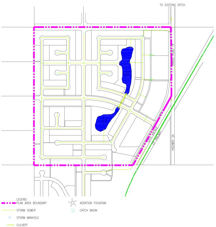
FIGURE 13.0 PRELIMINARY STORMWATER DESIGN
