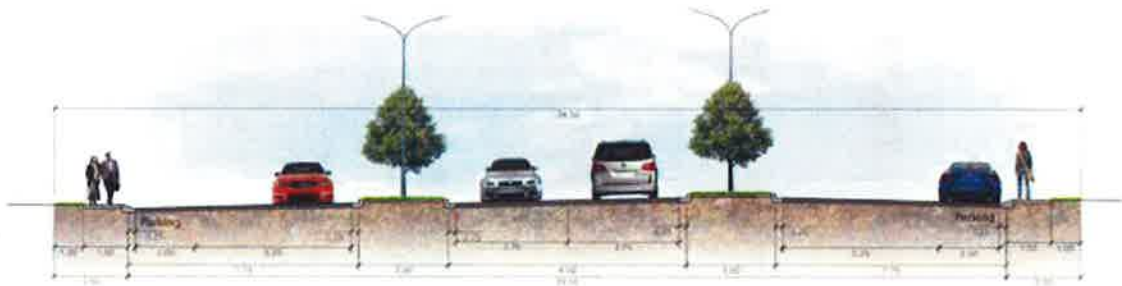
B-B: William Avenue - 42.5m / 34.5m Modified Collector Roadway 34.5m Portion of Roadway
